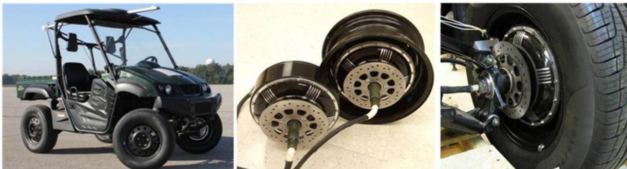
Fig. 1. EGV and the installed in-wheel motors.
